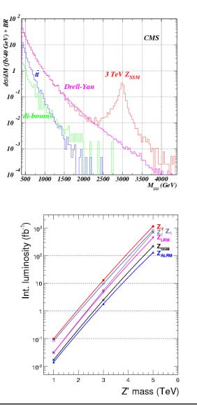
Cross section times the branching ratio for 3 TeV Z' of the Sequential Standard Model (red) as a function of the  $\mu+\mu$ invariant mass  $M\mu\mu$ , compared with the production of muon pairs in a few main background sources.
