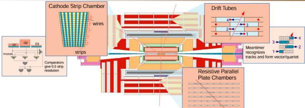
CMS uses three types of gaseous particle detectors for muon identification Drift Tubes (DT): central barrel region ( $|\eta| < 1.2$ )
