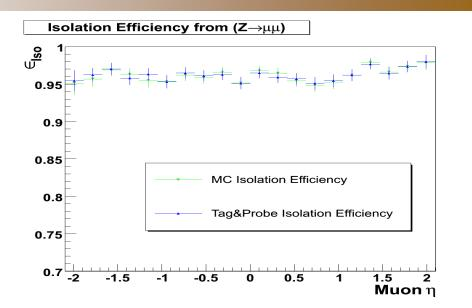
Efficiencies from Tag-and-Probe method are compatible with efficiencies calculated from Monte Carlo studies
